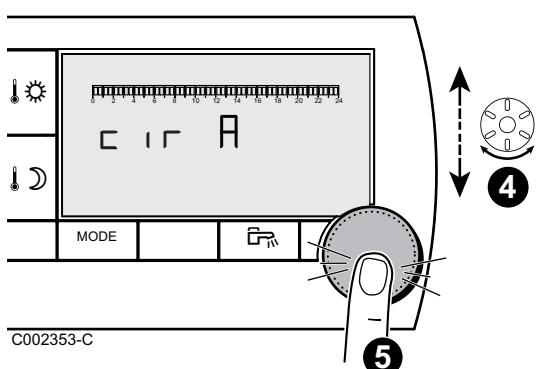
**4** Turn the settings button to select the desired circuit.
