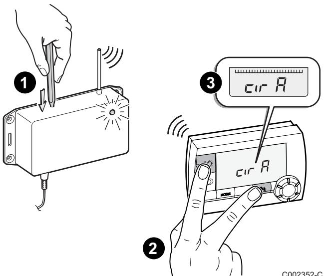
**1** Press the button on the radio module using the tip of a ballpoint pen. The light on the radio module comes on.
